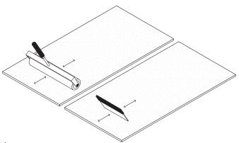
We strictly recommend product levelling after glue installation, to remove all air bubbles. Levelling is suggested in two phases, first with manual pressing, then with a heavy duty floor roller.
